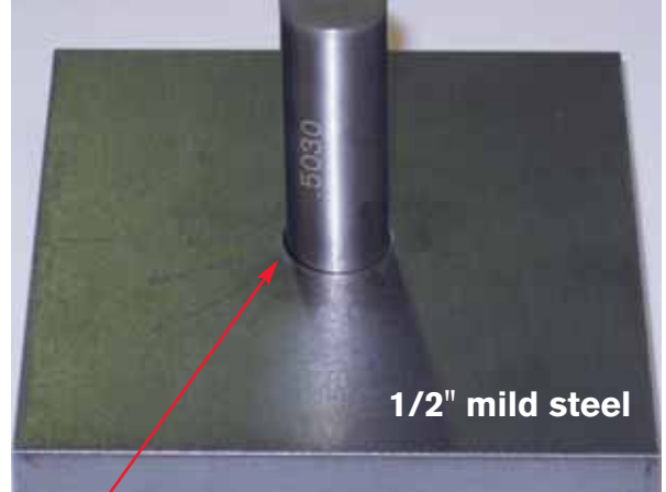
1/2" hole with True Hole technology cut with HPRXD® Plasma
