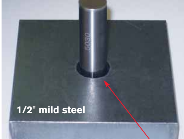
1/2" hole without True Hole technology cut with HPRXD® Plasma
